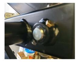
Note: It is important that pins and bushings should still be inspected for wear or damage per the normal suggested maintenance schedule.
