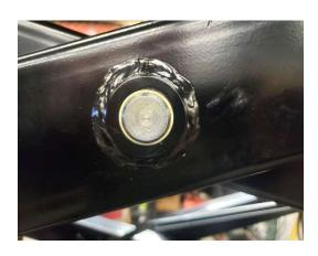
Along with the greaseless bushings, Skid-Lift has locked the pin from movement on the inner arms further reducing any possibility of wear of the inner arms. This means that pin rotates only on the wear bushings or the plastic slide blocks at the top of the bottom of the lift. This can be seen in the photos below:
