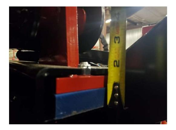
Caution! Failure to inspect slide blocks and replace as needed can result in the basket or scissor stack to feel loose in the slide block tracks. If not addressed properly, this could cause binding and/or slide block attachment bolts to catch on the slide rail during operation of the lift which could result in damage to the machine or serious injury to the user.
