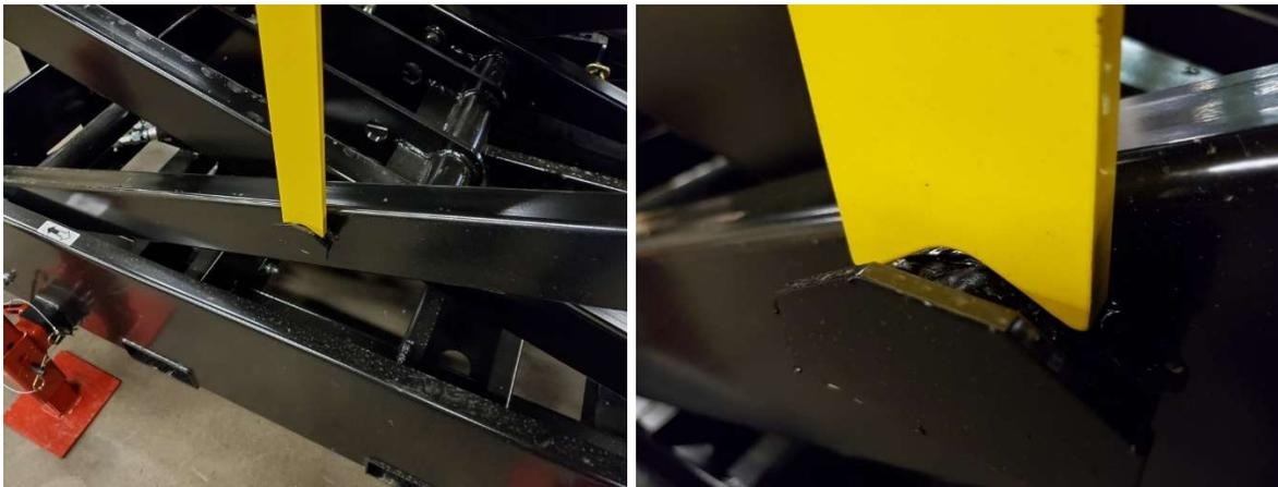
While the lift is in the up position on the maintenance bars, double check that all snap rings are in place and have the same amount of gap in the snap ring which will mean that all snap rings are seated properly.
